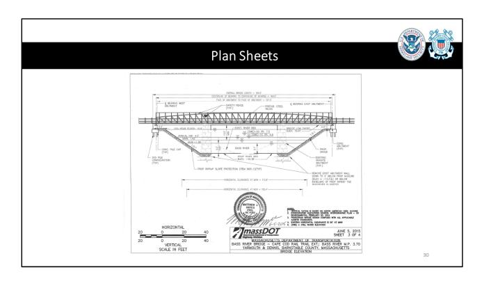
Here is an example of what we are looking for with it comes to plan sheets. As you can see here, this sheet shows the navigational clearances above the appropriate water surface elevations and the 100-year flood elevation. You can see the graphic bar scale and the title block showing sheet 3 of 4. These are just a few things listed on our plan sheet job aid, and Allen will dig deeper into plan sheets as well as the job aid later on today.
